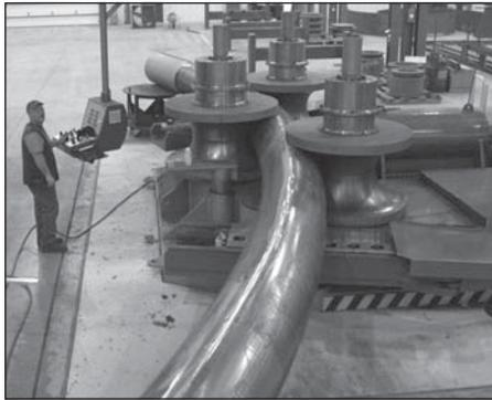
**Fig. 1. Bending of steel pipe in the production of pipe-bends for main pipelines**
