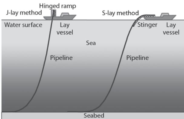
**Fig. 2. The bending of pipes under S- and J- method of main pipeline's laying on the seabed**
