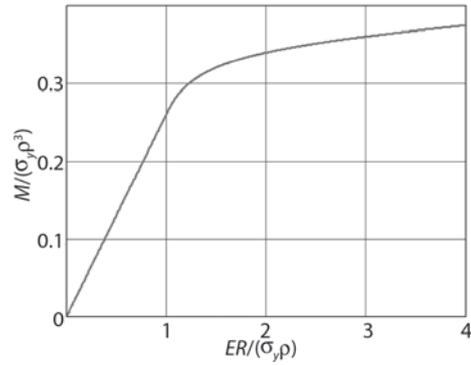
Fig. 6. The dependence of bending moment  $M$  from pipe's curvature  $1/\rho$
