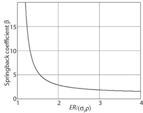
Fig. 7. The dependence of springback coefficient  $\beta$  from pipe's curvature  $1/\rho$
