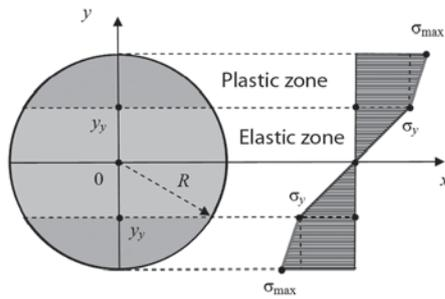
Fig. 5. The epure of the normal stresses in the cross section of round beam under bending
