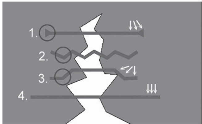
Fig. 4. Influence of different types of wire fiber on crack resistance: 1 – cone anchors fiber; 2 – wavy fiber; 3 – crooked ends fiber, 4 – straight fiber (blue circles – mechanisms of fiber anchoring, white arrows – adhesion surfaces)
