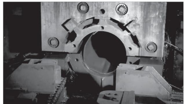
**Fig. 4 Bending of steel pipe billet on the final-shaping press of TEWA 1020**
