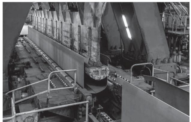
**Fig. 2. The pre-shaping press TEWA 1020 for bending the central region of steel sheet**
