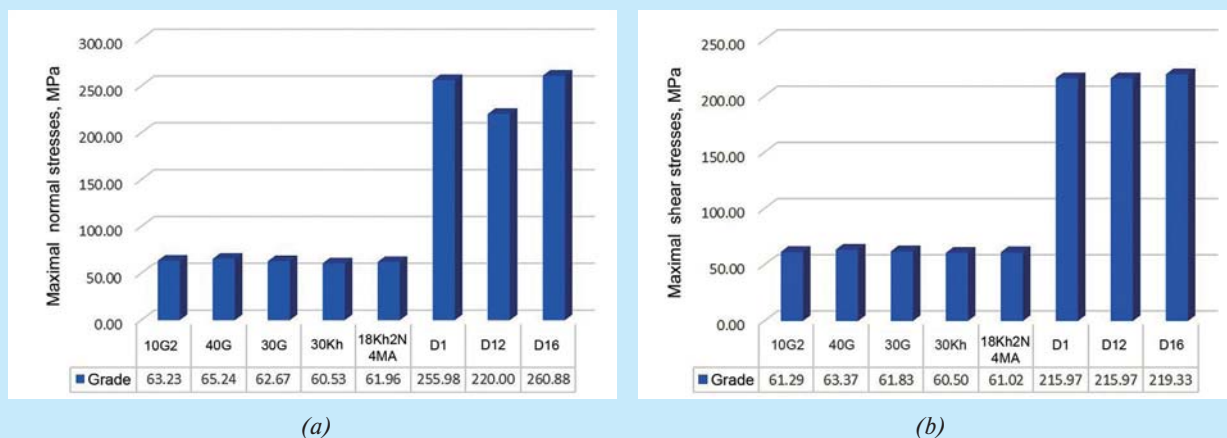
Fig. 4. Histograms of maximum values of the studied parameters at the joints of structures: a) normal stresses, MPa; b) shear stress, MPa
