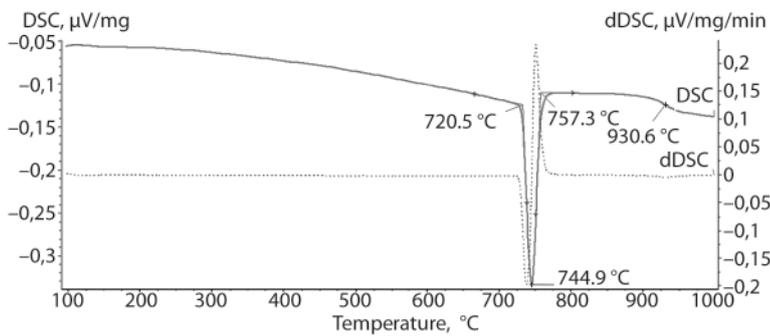
**Fig. 1.** DSC curve and DSC derivative curve (on time) for continuous heating of hot-rolled steel 80 with rate 10 °/min
