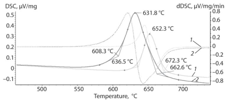
**Fig. 3. DSC curve and DSC derivative curve (on time) for continuous heating of hot-rolled steel 80:**
