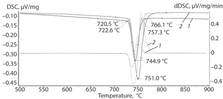
**Fig. 2.** DSC curve and DSC derivative curve (on time) for continuous heating of hot-rolled steel 80:
