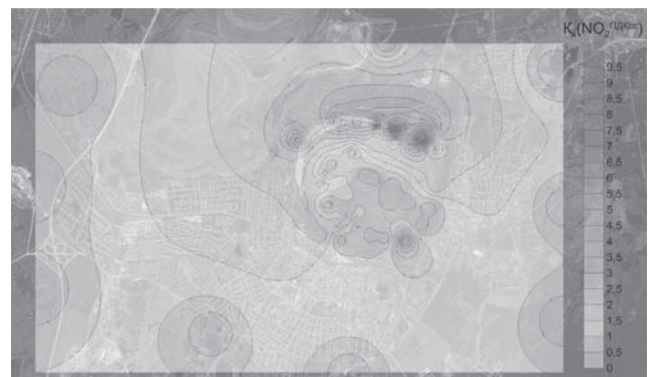
Fig. 4. Chemical envelope of contamination in the lowest atmospheric air with nitrogen dioxide from unmanned aircraft measurements
