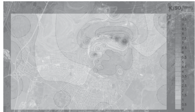
Fig. 3. Chemical envelope of contamination in the lowest atmospheric air layer with sulfur dioxide from unmanned aircraft measurements
