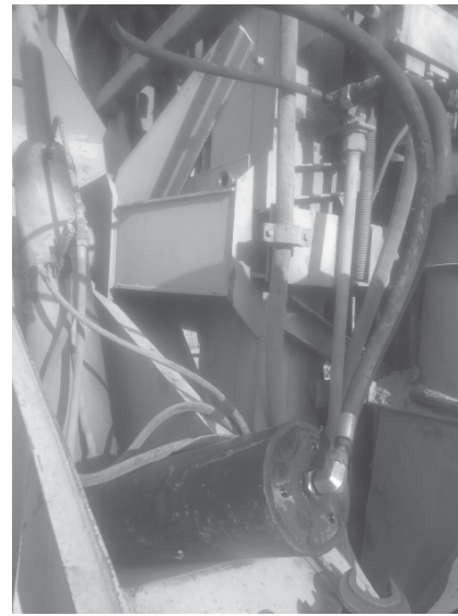
Fig. 2. Connection of hydropneumatic accumulator to main line of redesigned feed cylinders of drill rig model SBSH-250MNA-32
