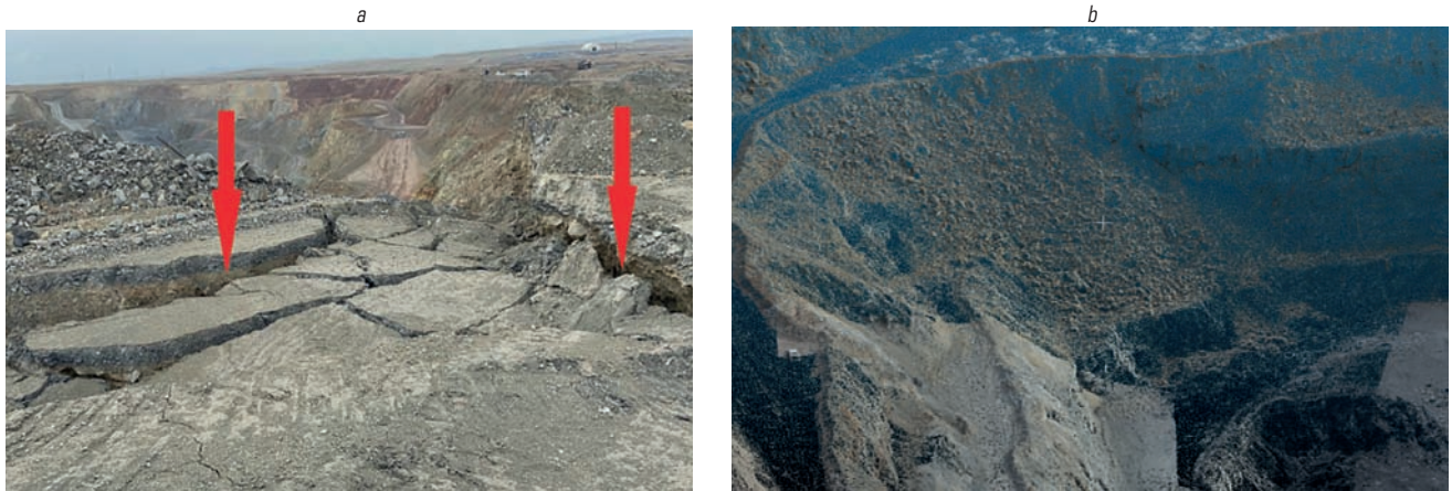
Fig. 4. Landsliding on eastern (a) and southern (b) pitwall at the Eastern Saryoba
