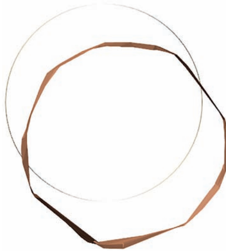
Fig. 6. Fracture in cast-iron tubing (level 88–89 in the shaft) and horizontal section at level 88 at elevation –145.275 m
