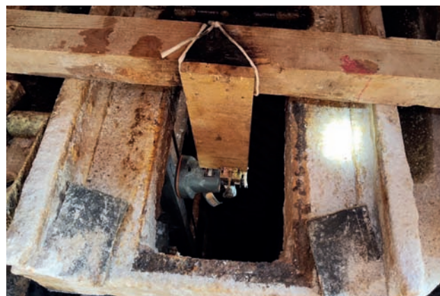
Fig. 1. Arrangement of SLAM CHCNAV RS10 scanner beneath the cage
