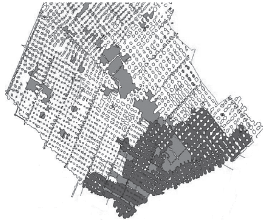
Fig. 1. Hydraulic fill of mined-out voids at safety pillar under the northern areas of the Zhezkazgan town
