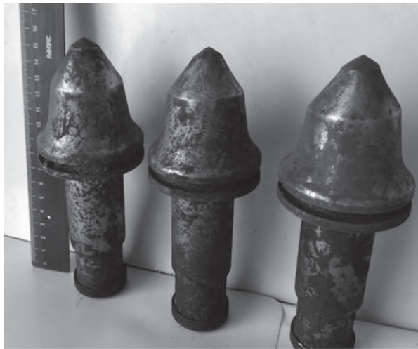
Fig. 4. Worn-out picks with remnants of hard-alloy tips
