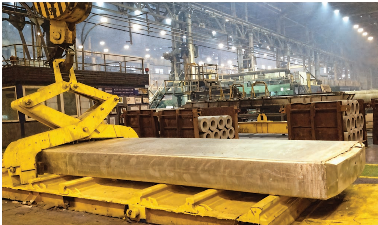
Fig. 1. Large-sized industrial ingot made of alloy 1580 (photo by authors)
