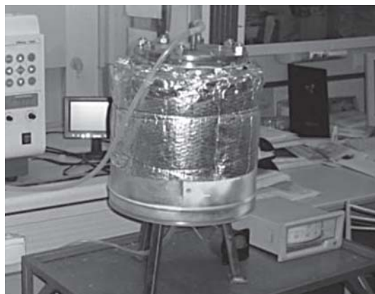
Fig. 2. Stainless steel installation for obtaining large portions (around 1 kg) of dispersed surface-modified metals (Ni, Cu, Fe)
