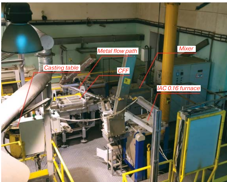
Fig. 2. Semi-continuous casting unit (photo by authors)
